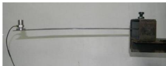
Figure Experimental Setup for Cantilever Beam
