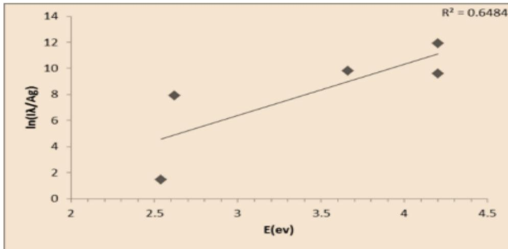
Figure 4. Boltzmann plot for (5) neutral spectral lines produced by the 1064 nm Nd:YAG laser irradiation with 140mJ
