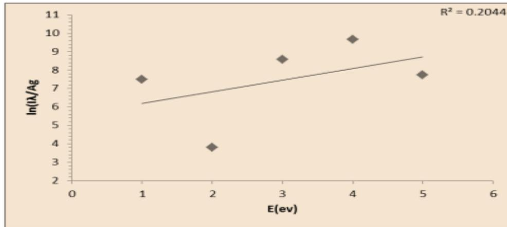
Figure 5. Boltzmann plot for (5) neutral spectral lines produced by the 1064 nm Nd:YAG laser irradiation with 200mJ
