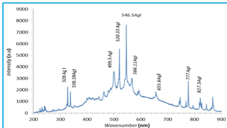
Figure 1. Emission profile of neutral versus ionized silvery plasma, created by a photons lamp at such a 5 millimeter distance mm, with 140 mJ total laser energy, encompassing the area with a spectral range of 200-900 wavelengths.
