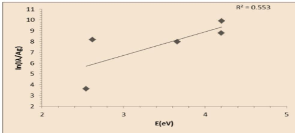
Figure 6. Boltzmann plot for (5) neutral spectral line produced by the 1064 nm Nd:YAG laser irradiation with 225mJ
