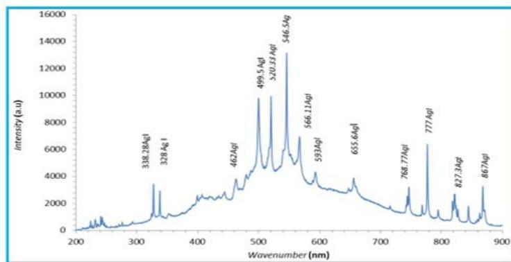
Figure 2. The emitted spectrum of free and ionized silvery plasma, created by such a 1064 nm light at a wavelength of 5 mm with 225 mJ pf laser pulses, encompassing the range of 200-900 wavelengths in the broad window
