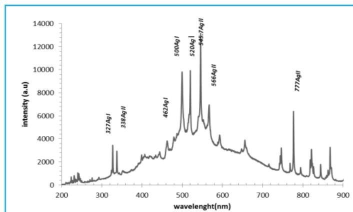
Figure 3. Emission pattern of neutral versus ionized silvery plasma created by a 1064 nm light at such a wavelength of about five mm, with a laser pulses of 200 michael jackson, encompassing the area with a spectral windows of 200-900 wavelengths.
