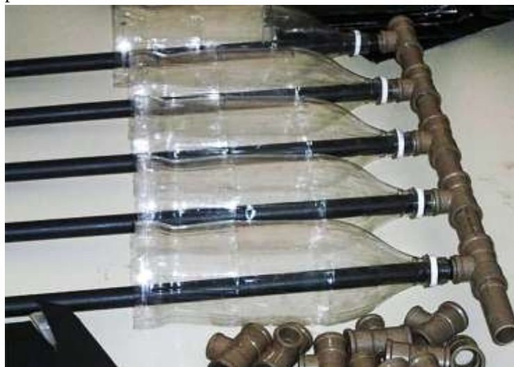
Figure: PET Solar Heating System
