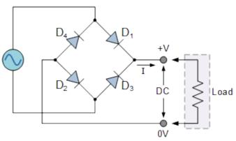
The four diodes labelled  $D_1$  to  $D_4$  are arranged in "series pairs" with only two diodes conducting current during each half cycle. During the positive half cycle of the supply, diodes D1 and D2 conduct in series while diodes D3 and D4 are reverse biased and the current flows through the load as shown below.
