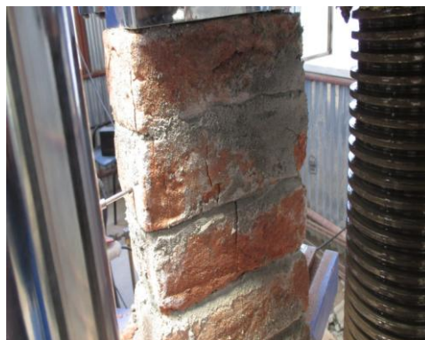
Fig 7: Failure pattern of 1.2 mortar grade sample placed submerged
