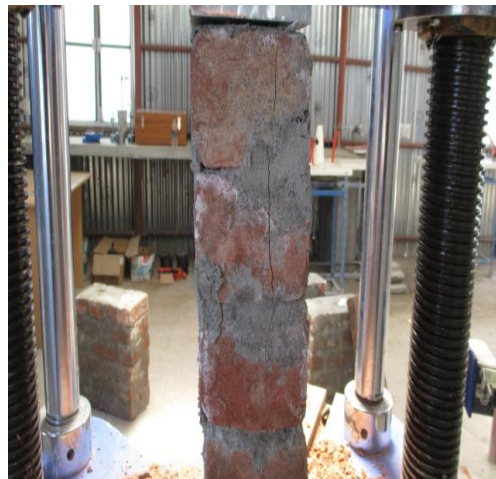
Fig 6: Failure pattern of 1.3 mortar grade sample placed submerged
