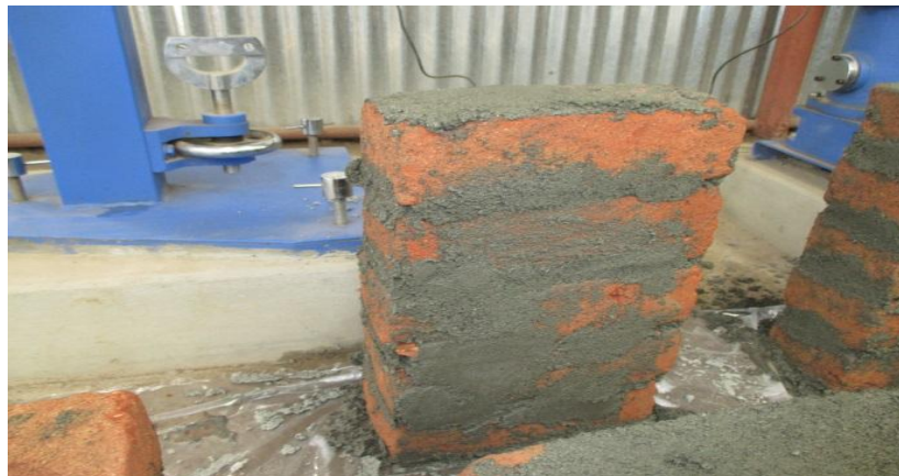
Fig 1 : Stricter face of sample undergoing compression
