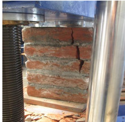
Fig 8: Failure pattern of 1.6 mortar grade sample placed submerged
