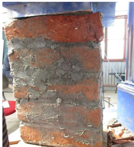
Fig 3: Failure pattern of 1.3 mortar grade sample after 7 days
