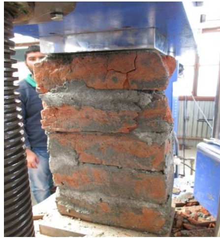
Fig 5: Failure pattern of 1.6 mortar grade sample after 7 days
