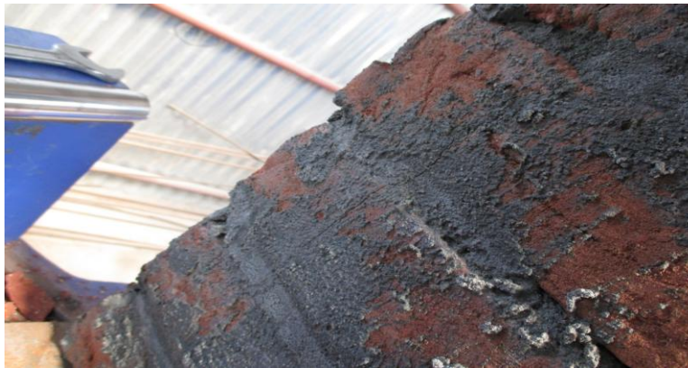
Fig 3: Failure pattern of 1.3 mortar grade sample after 7 days
