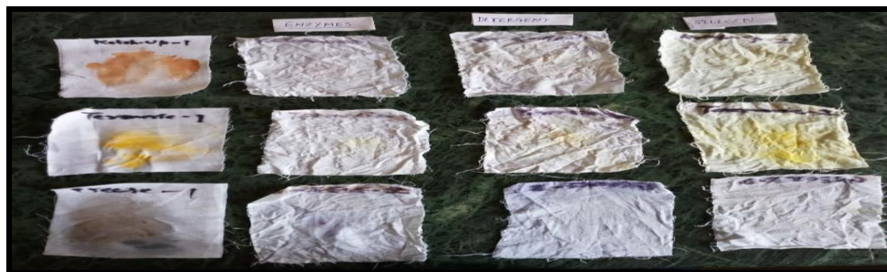
Fig :washing behavior of stained cotton cloth with ketchup, turmeric and grease and washed with three types of washing agent detergent, enzymes and silicon.
